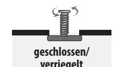
VENTILSTIFT OBEN = VENTIL GESCHLOSSEN
