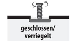
VENTILSTIFT OBEN = VENTIL GESCHLOSSEN
