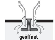
VENTILSTIFT UNTEN = VENTIL GEÖFFNET
