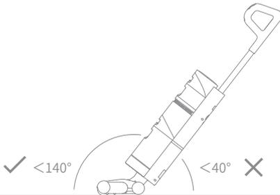
Do not recline the vacuum more than  $140^\circ$  to protect against water leakage.
