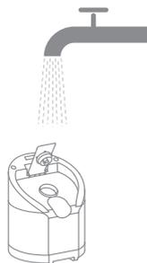
3. Tightly close the tank cover after the water has been added.
