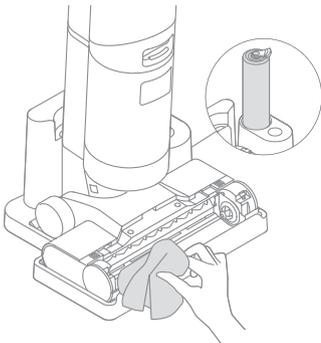
4. After cleaning is completed, align the right end of the roller brush with the vacuum and push the left end into the left slot on the vacuum until it clicks into place.
