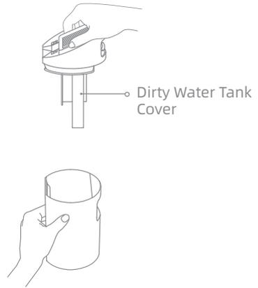
3. Rinse the tank and tank cover with clean water. Clean the inner wall of the tank with the included cleaning brush.
