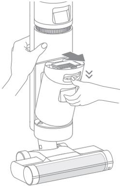
2. Hold the tank with one hand and pull up the tank cover with another hand to pour out the dirty water.
