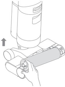
2. Use the included cleaning brush to remove hairs and debris that get stuck in the roller brush and rinse it with clean water. The roller brush must be thoroughly dried before use.
